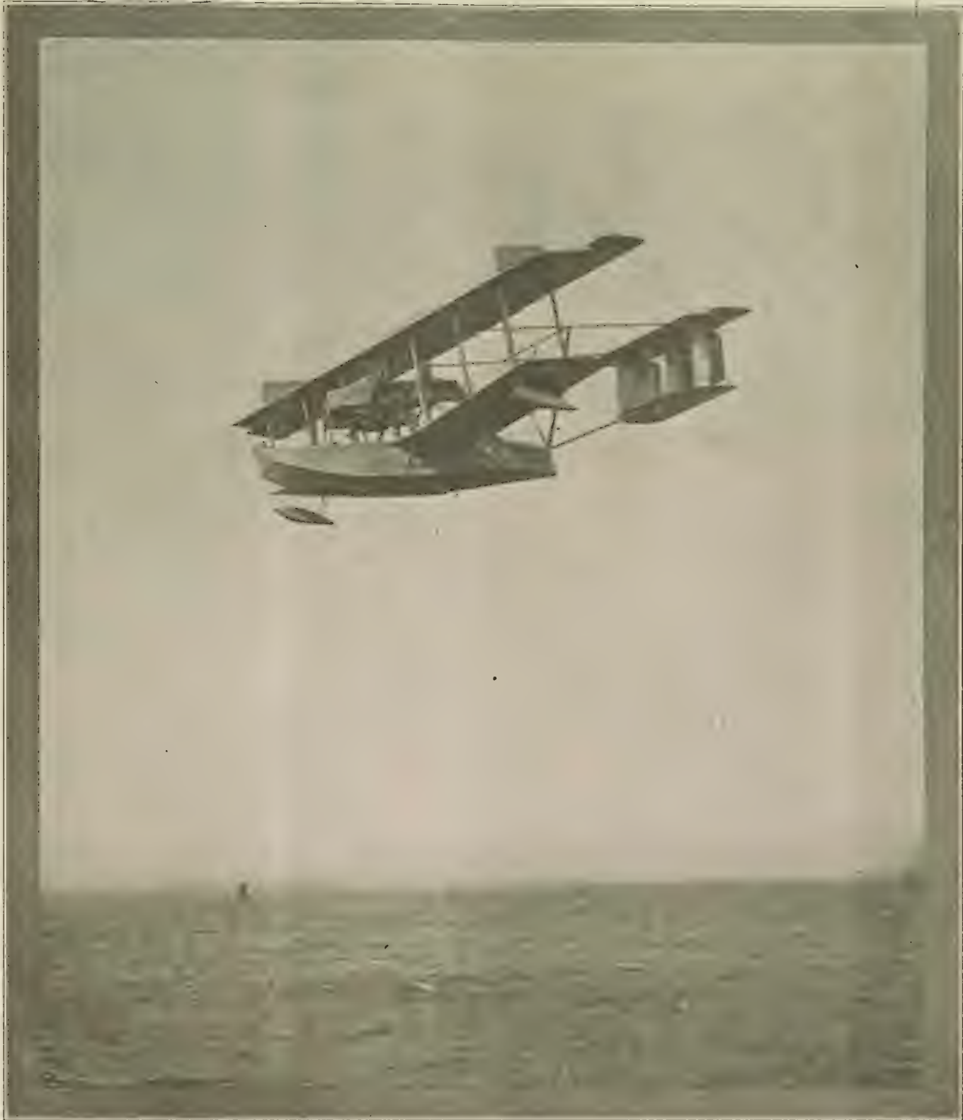
The Four-Engined NC-2 Which Is Soon Expected to Fly Across the Atlantic. The Liberty Engines Are Mounted in Tandem on Either Side of the Body
